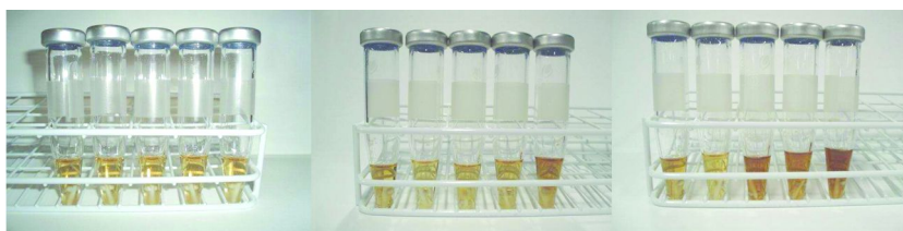
Figure 9. Dissolution of cellulose in [EMIM]Cl under microwave irradiation: a) 6 wt-% of cellulose, 100 °C, power between 60 and 140 W, 30 min; b) 2–10 wt-% of cellulose, 140 °C, 80 W, 30 min; c) 2–10 wt-% of cellulose, 160 °C, 80 W, 30 min.
