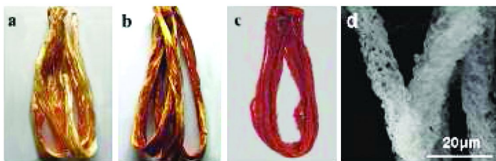
Figure 8. Photographs of the cellulose/ \text{Fe}_2\text{O}_3 nanocomposite fibers of F001 (a), F01 (b), and F05 (c) with different \text{Fe}_2\text{O}_3 contents, as well as fiberlike \text{Fe}_2\text{O}_3 nanomaterials calcinated from F05 (d) (54).
