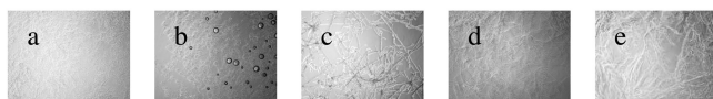
Figure 3. Structures of cellulose regenerates – a cellulose xanthogenate/caustic soda, regenerated from aqueous sulphuric acid - irregular ; b – cellulose acetate/acetone, regenerated from water – irregular/fibrous; c – cellulose/cuoxam, regenerated from water – fibrous; d – cellulose/NMMO / H 2 O, regenerated from water – fibrous; e – cellulose/BMIMCl, regenerated from water – fibrous
